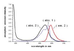
The blue line (abs. 1) represents the absorption spectrum of the free label, the black line (abs. 2) the conjugated form. The red line (em. 2) shows the fluorescent emission spectrum of the conjugated Chromeo P543.
