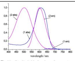
The blue line (1 abs) is the absorption spectrum of free label, the red line (2 abs) of the conjugated form. The blue line (1 em) is the emission spectrum of free label, the red line (2 em) of conjugated Chromeo P503.
