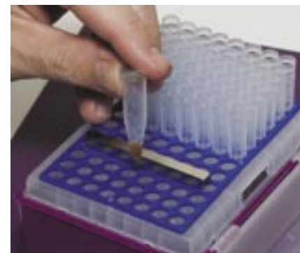
Figure 2: Use of a standard tip box for magnetic ChIP. ChIP-IT Express Kits include a strong bar magnet that can be used to convert tip boxes into a magnetic stand for washing the protein G-coated magnetic beads.
