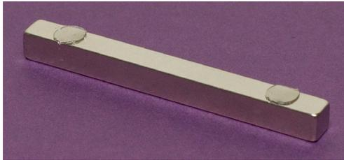
3. Remove the covering tape from the exposed side of the glue dots. Fix the magnet to the tip box so that it is against the PCR tubes. The magnetic stand is now ready for use.
