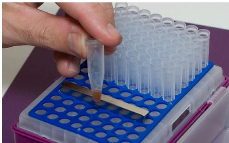
3. Allow the beads to pellet completely and remove supernatant with a 1000  $\mu$ l pipette. You can either leave the tube in the rack or pull it out when you remove the buffer. The beads will remain on the side of the tube, even when not next to the magnet.
