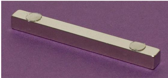
4. Remove the covering tape from the exposed side of the glue dots. Fix the magnet to the tip box so that it is against the PCR tubes. The magnetic stand is now ready for use.
